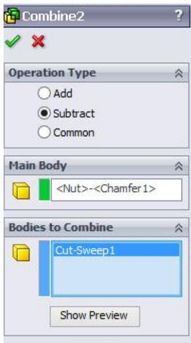
**11.Insert>Feature>combine>** Select Main body of nut and bolt >OK and save the file with different name.
