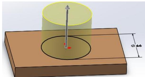
4.extrude to 50 mm (Select the face by (Enter Space bar> double click the plane) and Draw the 2D sketch as given above
