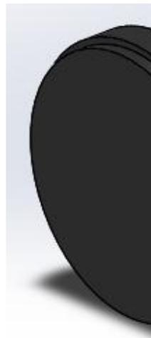
Create circle of 2D sketch as per the dimensions, on right plane and extrude to 20mm (Select the face by (Enter Space bar> double click the Normal plane) and Draw the 2D sketch as given above. Extrude by (Insert>Boss/Base>Extrude)) ok.
