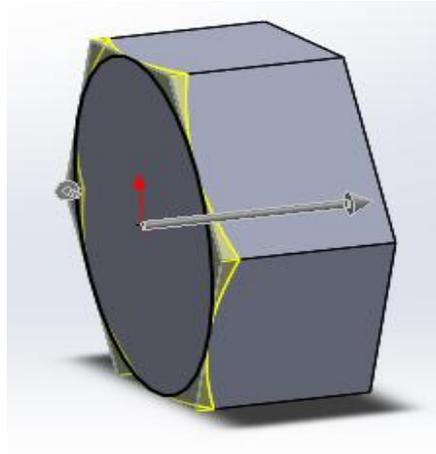
5. Create circle of 2D sketch of Diameter of 11.6 mm, on right plane and extrude cut to 7mm taper 60°, flip side to cut, draft inward. (Select the face by (Enter Space bar> double click the Normal plane) and Draw the 2D sketch as given above. Extrude cut by (Insert>Boss/Base>Extrude)) ok.
