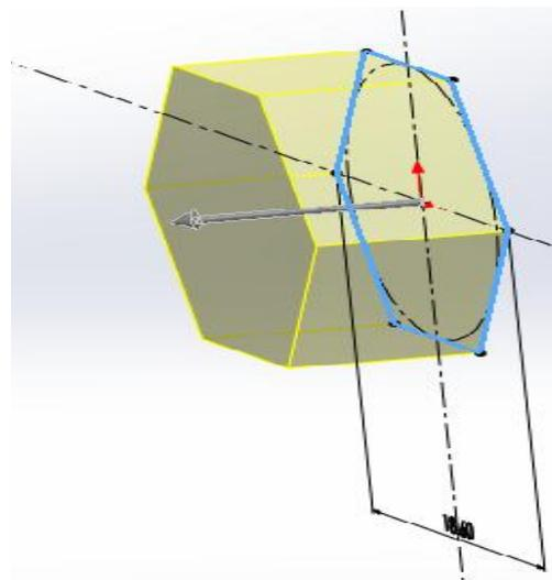
4. Create circle of 2D sketch of Hexagonal width of 11.6 mm, on right plane and cut extrude to 7mm, (Select the face by (Enter Space bar> double click the Normal plane)
