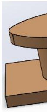
1. Use Extrude cut with dimensions of 42 mm size circle as per below figure.
