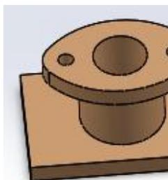
Create a hole as per the dimensions of 12mm size both sides.
