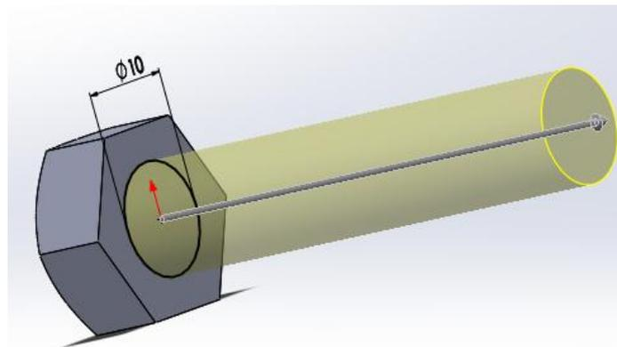
6. Create circle of 2D sketch of Diameter of 10 mm, on right plane and extrude to 7mm (Enter Space bar> double click the Normal plane)
