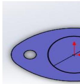
Extrude to 45 mm (Select the face by (Enter Space bar > double click the plane) and Draw the 2D sketch as given above, Extrude cut use through all. (Select the face by (Enter Space bar > double click the plane) and Draw the 2D sketch as given below,
