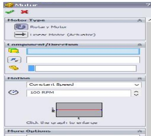
Start the motor> select the linear motor>motor location(select nut face ) and component to move relative to(select bolt ) ,motion at constant speed of 10mm/s>OK. Calculate and play.
